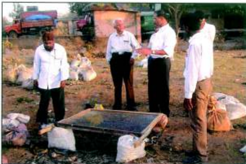
Photo 4.13 : 10mm size scive used for separation of MSW.
