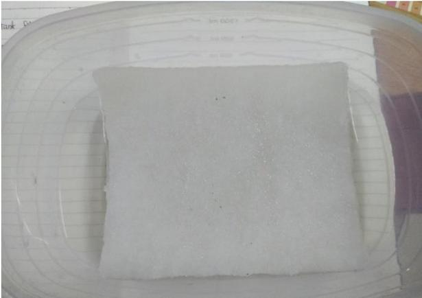
Fig 22 a: setup of 13\*11cm cut filter submerged in 320ml BG11 and 40ml inoculum
