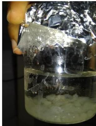
Fig 23: Microalgae trapped in calcium alginate
