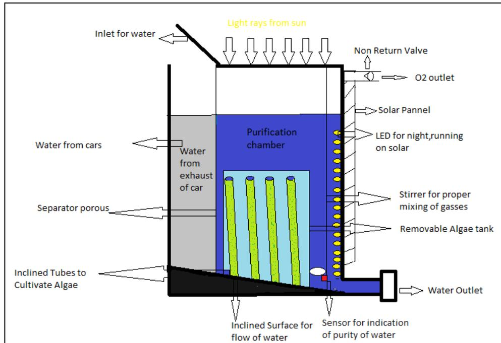
**Fig 26: Biofilter Design 1**
