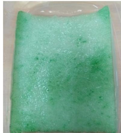
Fig 22 b: Immobilization of microalgae observed on the matrix
