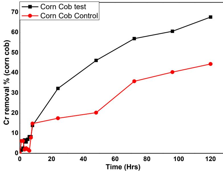
**Figure 52:** Graphical representation of the percentage chromium removal by corn cob with bacterial consortium and without bacterial consortium.
