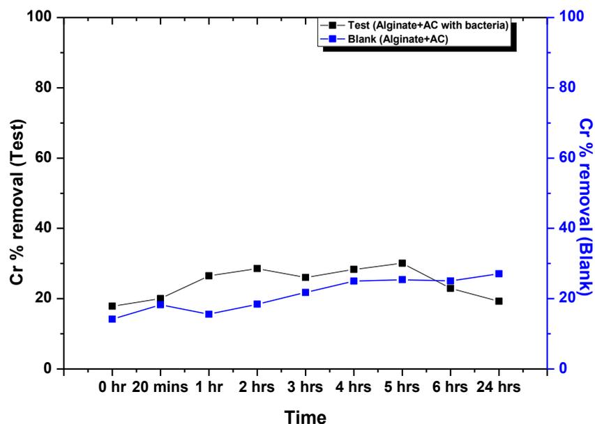
**Figure 41:** Chromium removal by the alginate and AC bead immobilized with Cr bacterial consortium and without bacterial consortium.
