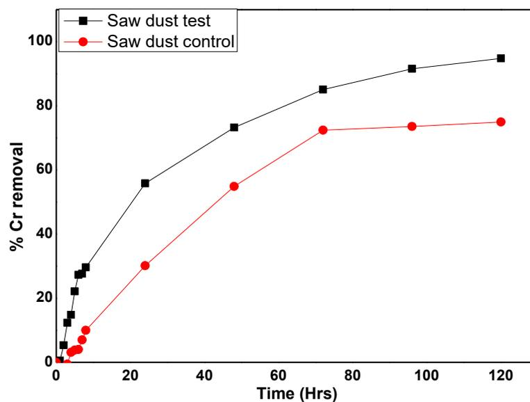
**Figure 54:** Graphical representation of the percentage chromium removal by saw dust with bacterial consortium and without bacterial consortium.
