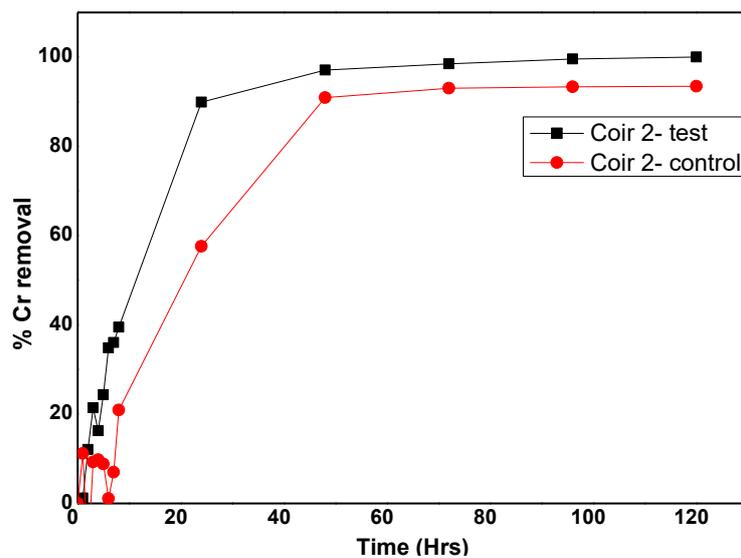
**Figure 48:** Graphical representation of the percentage chromium removal by coir with bacterial consortium and without bacterial consortium.
