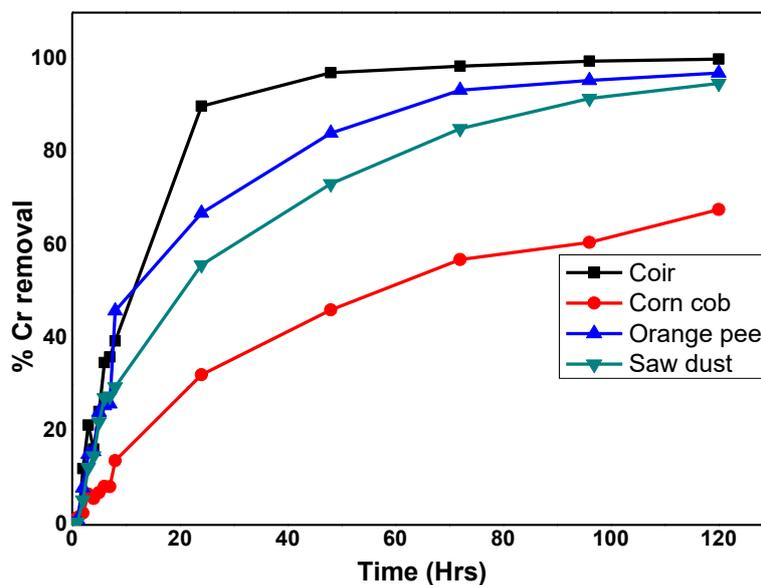
**Figure 55:** Graphical representation of the chromium removal by different biological waste immobilized with bacterial consortium.
