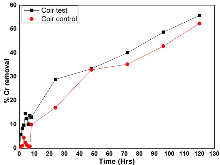
**Figure 46:** Graphical representation of the percentage chromium removal by coir with bacterial consortium and without bacterial consortium.
