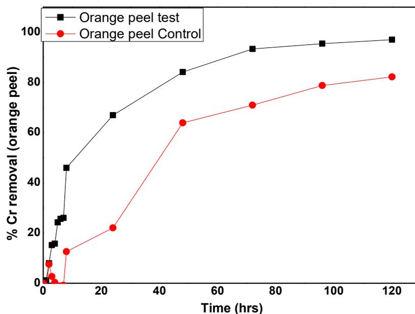
**Figure 50:** Graphical representation of the percentage chromium removal by orange peel with bacterial consortium and without bacterial consortium.
