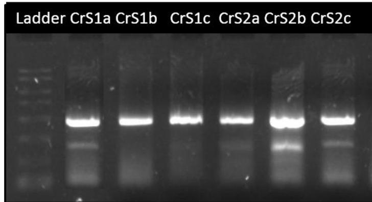
**Figure 9:** Agarose gel image of the 16S rDNA amplified product of chromium resistant bacteria.
