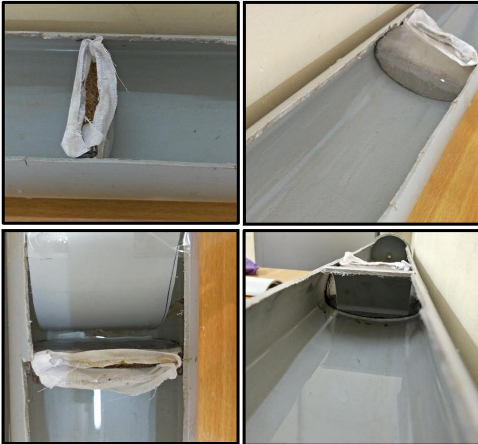
**Figure 59:** Image of biomat and baffles placed in the river model system for chromium treatment.
