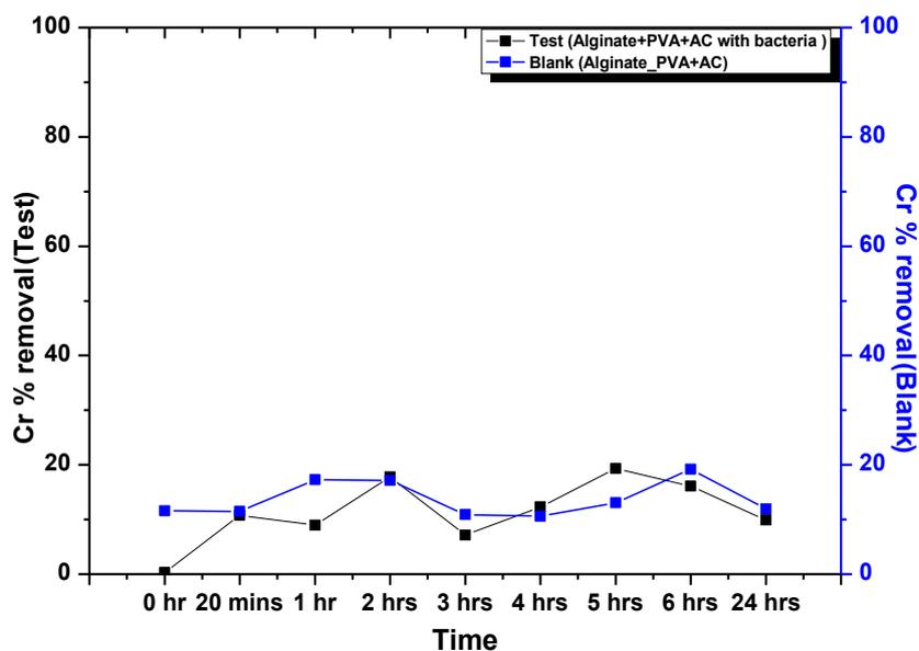
**Figure 42:** Chromium removal by the alginite, PVA and AC bead immobilized with Cr bacterial consortium and without bacterial consortium.
