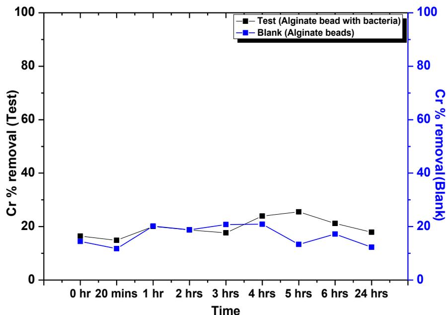
**Figure 39:** Chromium removal by the alginate bead immobilized with Cr bacterial consortium and without bacterial consortium.
