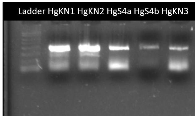
**Figure 10:** Agarose gel image of the 16S rDNA amplified product of mercury resistant bacteria.
