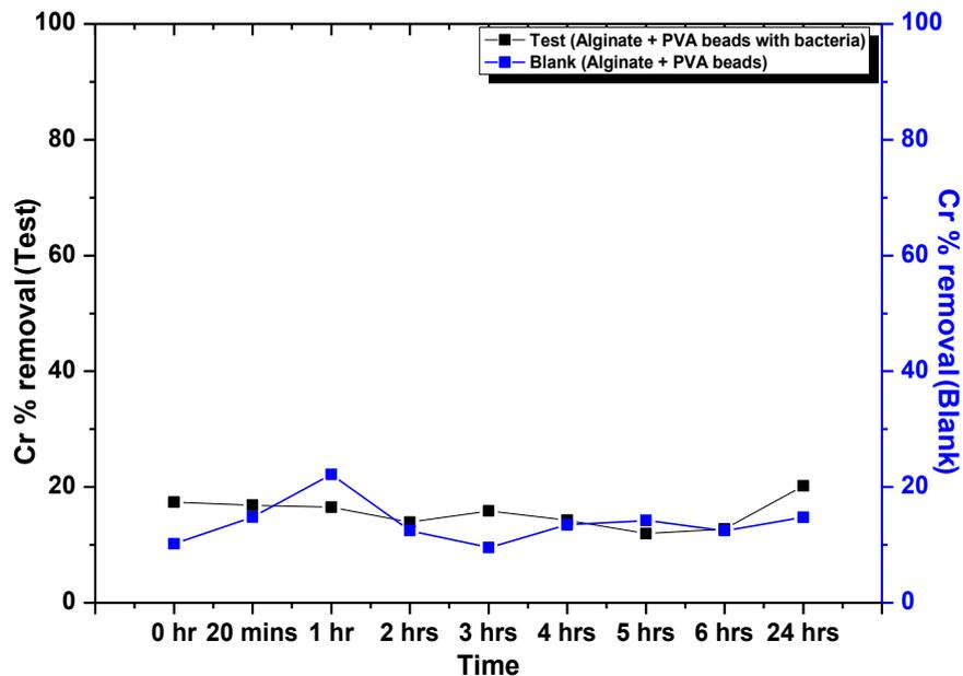
**Figure 40:** Chromium removal by the alginate and PVA bead immobilized with Cr bacterial consortium and without bacterial consortium.
