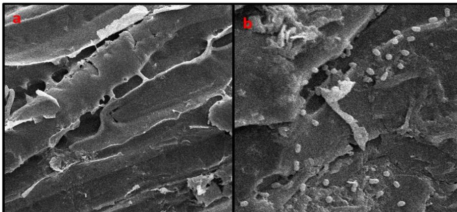
**Figure 47:** SEM image of Cr consortium immobilized on the coconut coir using another method (b) and control without immobilized bacteria (a).
