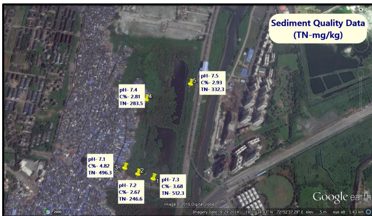
Figure 5.22: Sediment Quality Analysis Data at the Various Sampling Point
