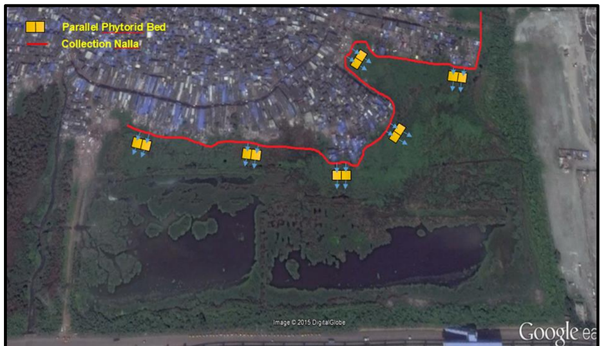
Figure 8.1: Representative Positioning of the Wastewater Treatment Plants
