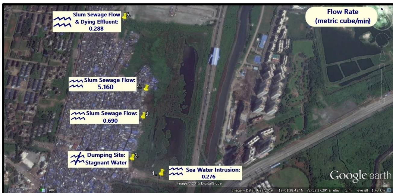
Figure 5.3: Flow Rate at Various Sampling Points
