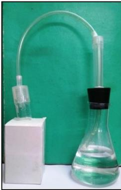
Fig 5. H<sub>2</sub>S setup
