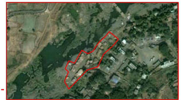
Encroachment of shacks into the river bed destroying natural edge vegetation. The floodplain of the river has not been determined and protected leading to development in these areas and annual flooding at Akloli.
