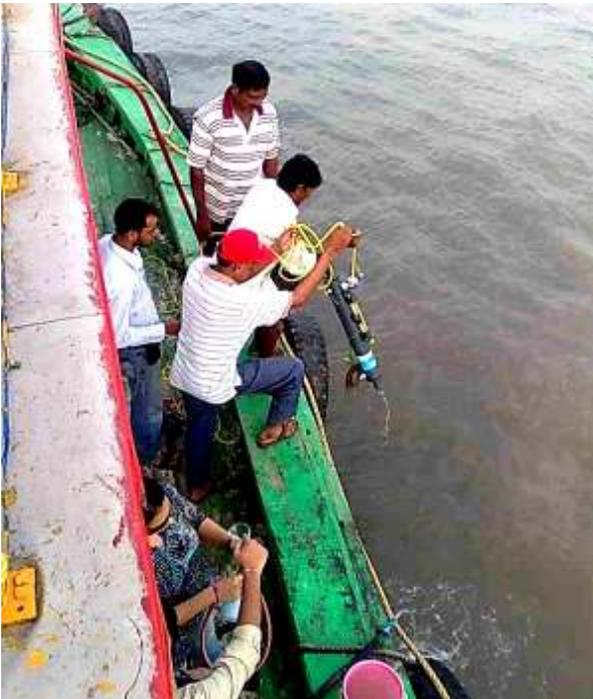
Water-sampler being deployed during cruise
