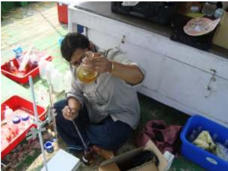
On-board measurement of dissolved oxygen
